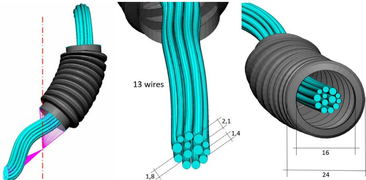
Fig. 1: Wire harness with bellow, axis of rotation, cable diameter, bellow diameter
