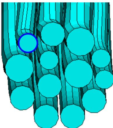
Fig. 2: Kinks from element facets, for contact original geometry should be recovered
