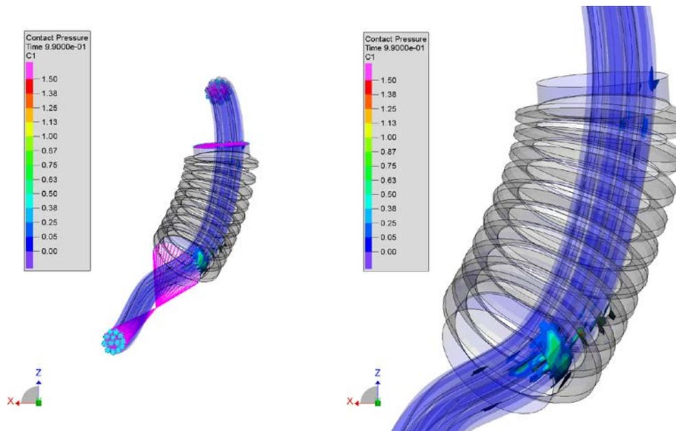
Fig. 3: Contact pressure at 70° door opening
