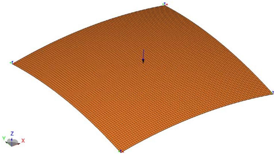
Figure 1: Boundary conditions and loads of a corner hinged shell
