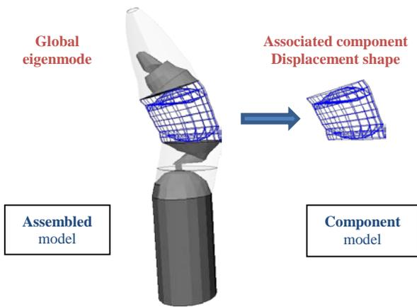
Figure 2. Loaded component mode
