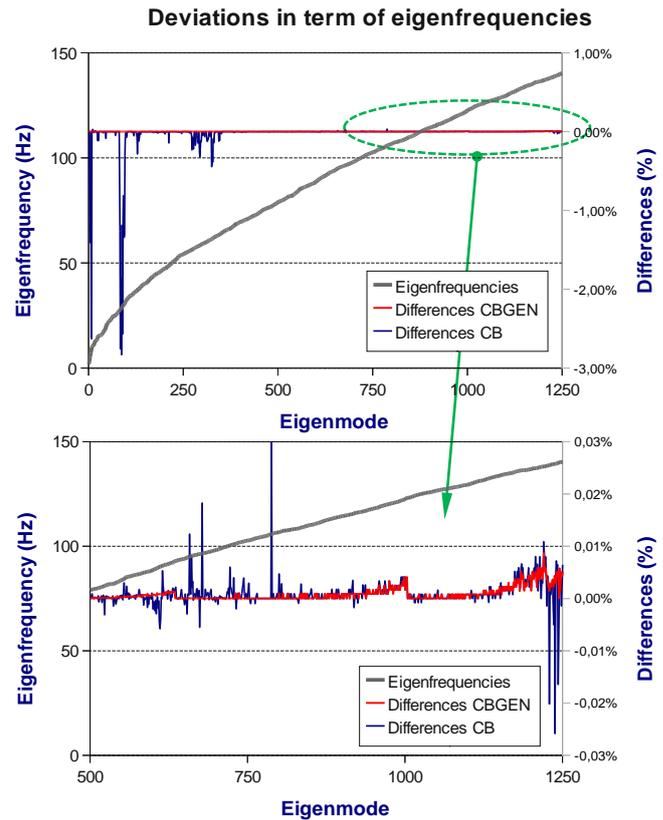
Figure 6. A5GS - Comparison between reduction methods
