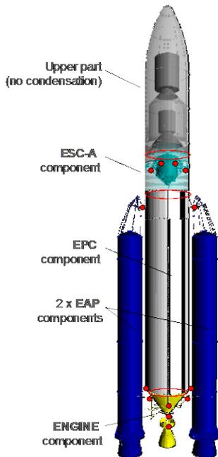
Figure 7. A5E/CA - Launcher reduction scheme
