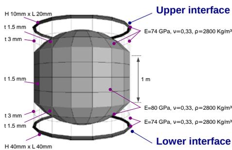
Figure 3. FE model of the dry tank
