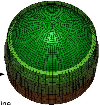
Shell property: handling of **thickness variation**. Possibility to split a section and affect various properties along a line (for example, to modelize circumferential welds)
