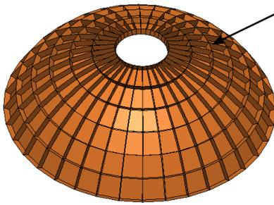
**Stiffeners system** for any type of surface (ribs, belts or orthogrids)
