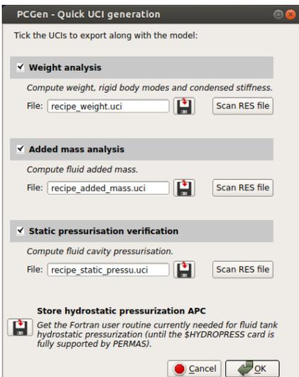
Generation of **UCI files** (with model complement) for some standard tests (such as weight analysis, hydrostatic pressurization check, added mass, rigid body modes decoupling, etc.)
