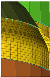
*In progress* **Volumic meshing** of thick parts, with handling of the solid-shell transition, and generation of the fluid interface and pressurization skins whenever needed.
