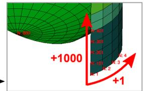
One minimum label, available for each object in PCGen, pilots the numbering of nodes, elements, local systems, lines and surfaces, and MPC definitions belonging to that object.
