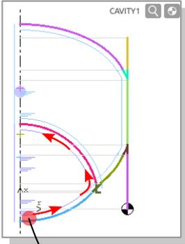
Automatic determination of the cavity envelope for a given a bottom
