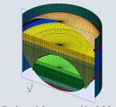
Tank model generated by PCGen Automatic node and element sets for different filling levels of tanks
