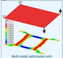
Multi-modal optimization with topology optimization, bead generation, and sizing optimization of sheet thicknesses
