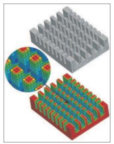
Analysis of cooling element with radiation
