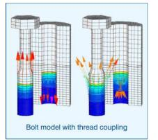
**Bolt pretension** is also made by contact. The coupling of screw and mating thread takes place at the thread area, while the bolt and the bolt hole remain perfectly cylindrical. By doing so, the radial widening of the bolt hole and the twist of the bolt can be modeled by a flank angle and the pitch of the thread without modeling the thread itself.
