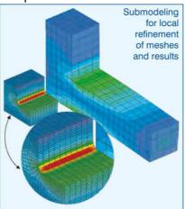
By **automated part coupling** through incompatible meshing of parts, more flexible and faster modeling is enabled, because meshes need not to be made compatible by expensive mesh adaptations and replacing parts by other meshes become much easier.
