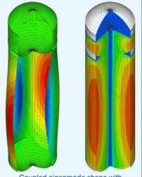
Coupled eigenmode shape with corresponding pressure distribution
