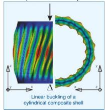
The linear **buckling** analysis is a classical method to study shell and beam structures. It can be used also after a nonlinear static analysis in order to detect additional bifurcation points.
