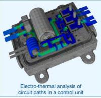
By **substructuring**, an FE model can be split into an arbitrary number of substructures (so-called components). The components can be assembled like single elements to get a complete structure (so-called configuration).
