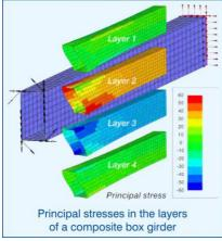
A special **spot weld element** is available, which essentially reduces the sensitivity of stress results due to the mesh size of the flanges.
