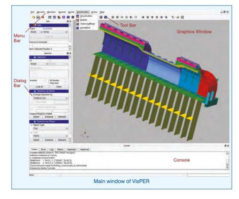
VisPER is the graphical preand post-processor of PERMAS. It comprises the pre-processing of PERMAS models (mainly on the basis of already existing meshes) and the post- processing of PERMAS results.
