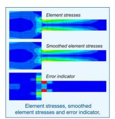
A Smooth Patch Recovery (SPR) method is applied to get **SPR stresses** beside classical stress calculation. The difference between both stresses defines an (Absolute) **Error Indicator** (AEI), which can be used for mesh validation and further mesh refinement, if required. In addition, the stress gradient normal to the surface is calculated at the surface nodes.
