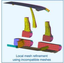
Results, which are calculated with a coarse mesh, can be applied as boundary conditions for a finer meshed part of the structure (e.g. in order to calculate more precise stresses). This **submodeling** technique also enables nonlinear analysis of parts based on linear analysis of the complete structure.
