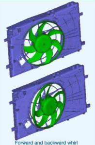
forward and backward whin of complex eigenmode shapes for a rotor in a non-rotating housing (by courtesy of MAHLE Behr GmbH & Co. KG)
