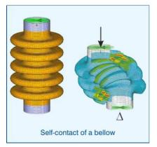
By **updating the contact geometry**, large sliding displacements can be calculated. Together with geometrical nonlinear effects, large rotations are carried out.
