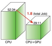
2\*Intel 6146(40core) Nvidia Tesla V100 GPU benefit for contact analysis
