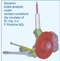
In **dynamic brake analysis** the contact status between brake pad and disc can be frozen for a subsequent real and complex eigenvalue analysis to identify instabilities indicating brake squeal. An additional parameter study using the integrated sampling method will give important hints on the brake's potential for improvement.
