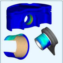
Optimization of the shape of a piston bore to reduce the edge pressure on piston pin (by courtesy of Mahle GmbH, Stuttgart)
