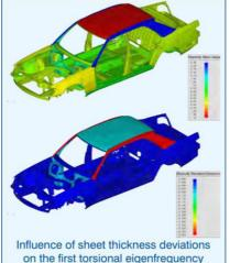
Due to the unification of optimization methods like parametric shape optimization, sizing and topology optimization, all these methods can be used simultaneously in a **Multi-Modal Optimization** to jointly solve an optimization task.
