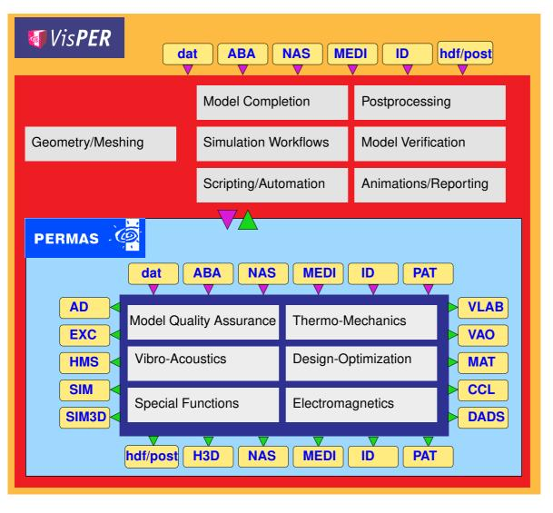
VisPER comprises PERMAS and uses the same data basis. So, a perfect data compatibility exists between pre-processing, analysis, and post-processing.
