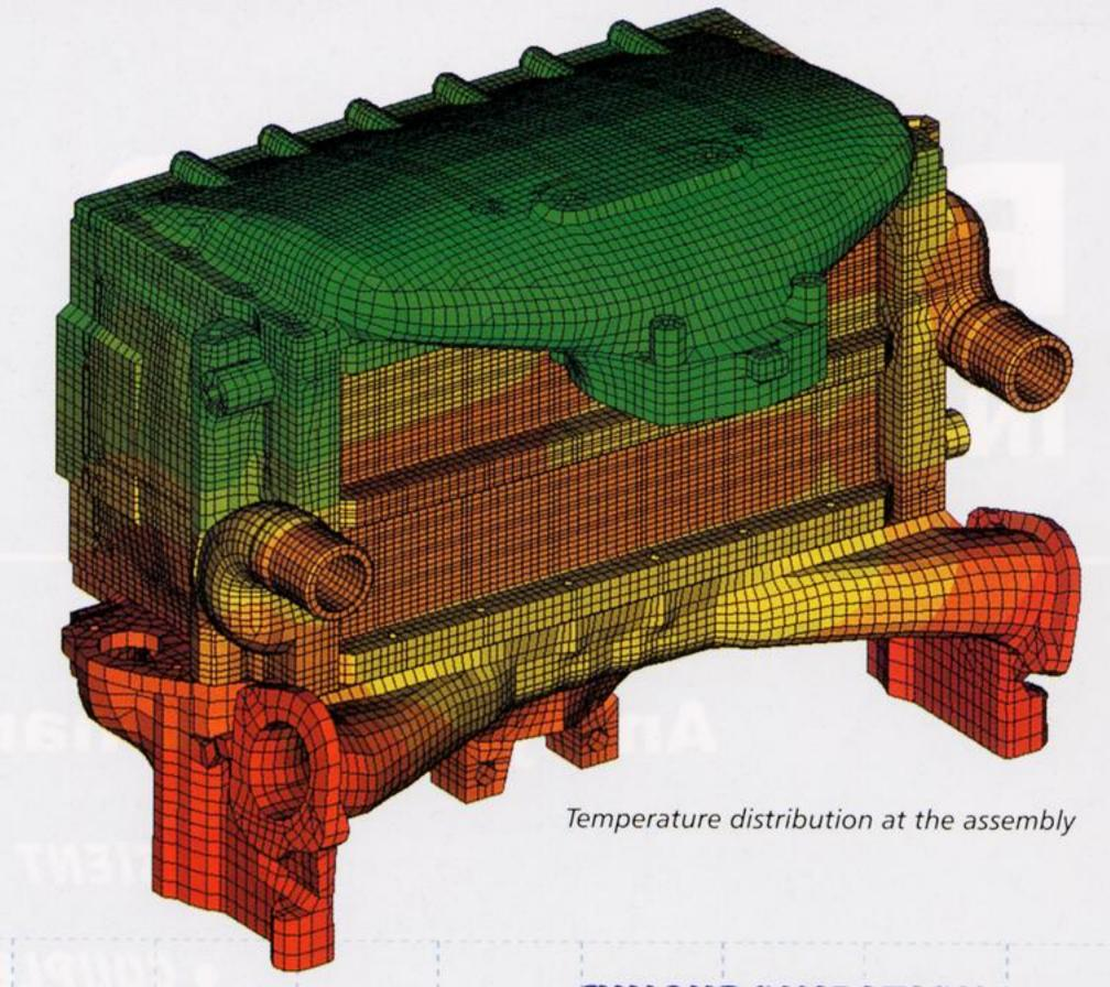
Contact definitions were first used to fix the top of the cooler to the case. Secondly, the prestresses of the screws were modelled correctly with contacts to represent the extensions of the bolts.
