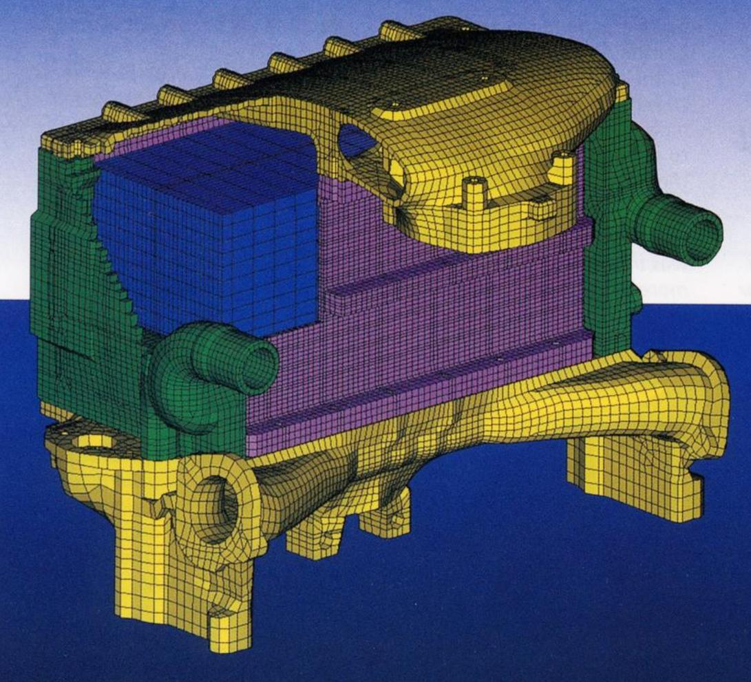
At Behr GmbH & Co., Stuttgart, a supplier of engine cooling and air conditioning for the automotive industry, complex structures are analyzed with PERMAS. The model parameters of this charge air cooler of BEHR Industrietechnik are impressive:
