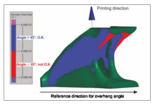
Figure 61: Check of overhang angle red: critical angle, blue: non-critical, other colors: no value (i.e. >90°).
