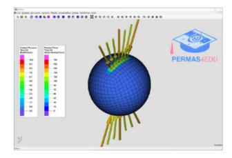
Figure 194: Contact pressures and forces
