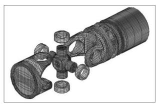
Figure 16: Model of a cardan shaft Voith Turbo GmbH & Co. KG, Heidenheim, Germany.
