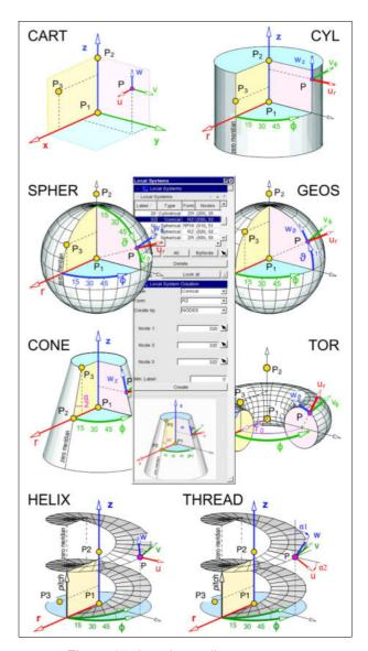
Figure 92: Local coordinate systems in VisPER
