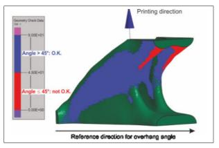
Figure 171: Check of overhang angle red: critical angle, blue: non-critical, other colors: no value (i.e. >90°).
