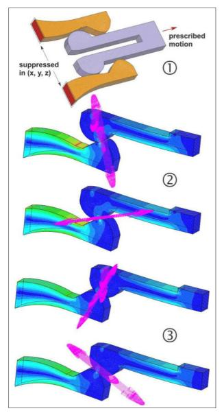
Figure 124: Clip example for contact update Large relative motion with friction. Picture 1 shows the model; pictures 2 show the contact pressure (above) and the frictional shear (below) with nodal point stresses before the bottleneck is reached; pictures 3 show the contact pressure (above) and the frictional shear (below) with nodal point stresses after the bottleneck is passed.
