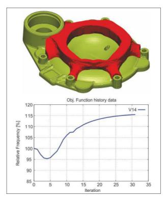
Figure 172: Topology optimization of a gearbox cover to maximize the second eigenfrequency with release direction (by courtesy of ZF Friedrichshafen AG)
