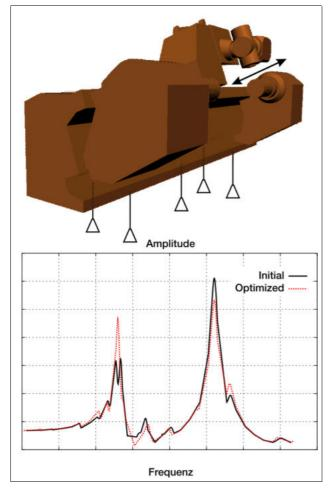
Figure 160: Frequency response optimization for a machine foundation where the position of the base spring elements is optimized which are coupled to the machine structure by interpolating surfaces. Design optjective is the lowest displacement of the tool center point.
