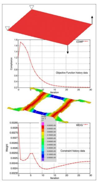
Figure 165: Multi-modal optimization with topology optimization, bead optimization, and free sizing for the sheet thicknesses.
