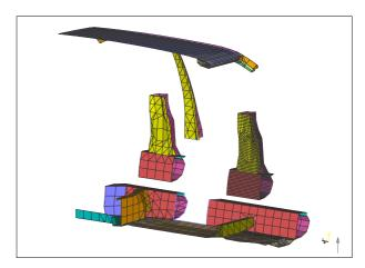
Figure 85: Application of local mesh refinement
