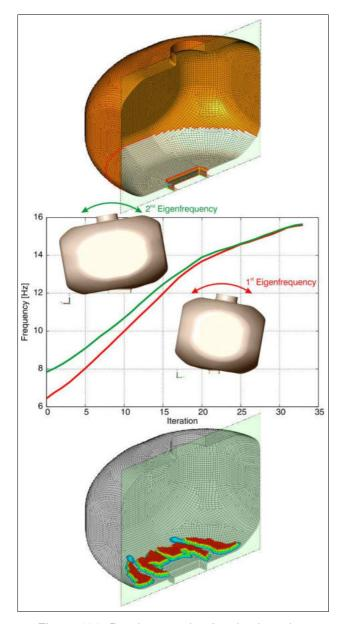
Figure 161: Bead generation for plastic tank
