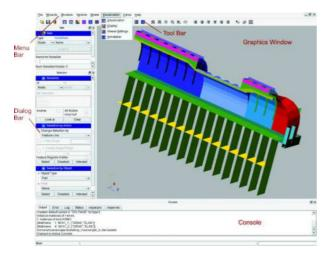
Figure 47: Main Window of VisPER
