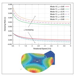
Figure 29: Simple brake model (3) with an unstable bending mode (m=2, n=1) which becomes unstable at different rotational speeds dependent on the frictional coefficient.
