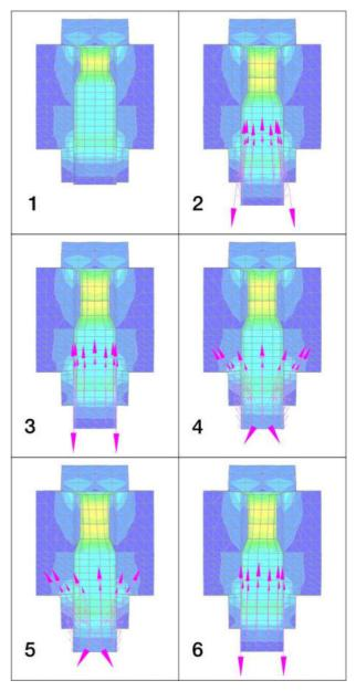
Figure 112: Bolt pretension
