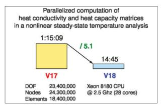
Figure 142: Parallelization of conductivity and capacity matrices.
