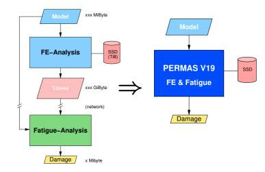
Figure 179: External and integrated fatigue work-flow
