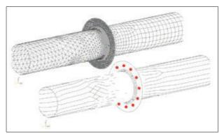
Figure 90: Spotwelds and incompatible meshes
