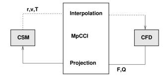
Figure 106: Coupling of CFD and CSM
