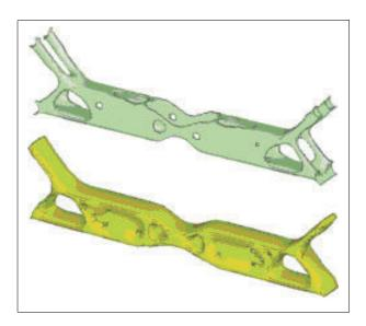
Figure 170: Different results for topology without (above) and with (below) release directions
