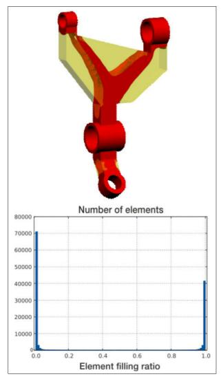
Figure 173: Fully converged topology
