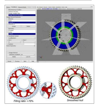
Figure 56: Topology optimization of a gearwheel Definition of cyclic symmetry and release directions, max. stress at interface between design space and gear rim, max. allowed weight, minimum compliance as objective function (by courtesy of Daimler AG, Stuttgart).
