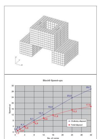
Figure 15: Static analysis with 3 loading cases 1.5M nodes, 176k HEXE27, 4.4M Dof run time on Intel Boxboro
