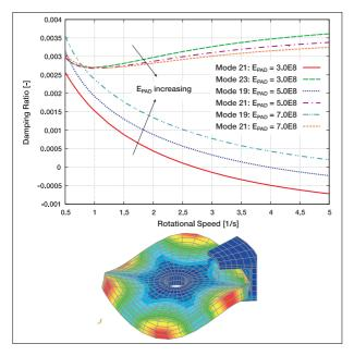
Figure 30: Simple brake model (4) with an unstable bending mode (m=3, n=1) which becomes unstable at different rotational speeds dependent on Young's modulus of the brake pad.
