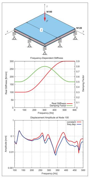
Figure 150: Frequency-dependent stiffness and frequency dependent viscous damping in frequency response analysis
