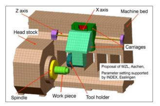
Figure 34: Simplified model of a turning machine as proposed by WZL in Aachen and supported by INDEX, Esslingen for setting suitable parameters
