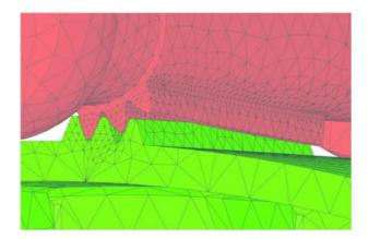
Figure 110: Contact with incompatible meshes
