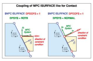
Figure 8: Surface coupling
