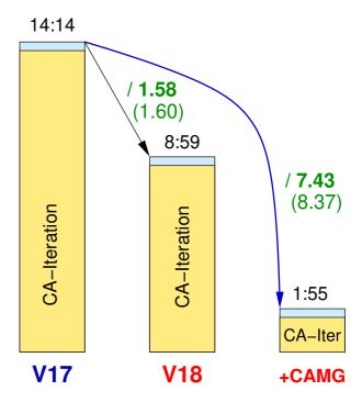
Figure 123: Computation time (hours) and speedup for large contact model for V18 and V18+CAMG compared to V17
