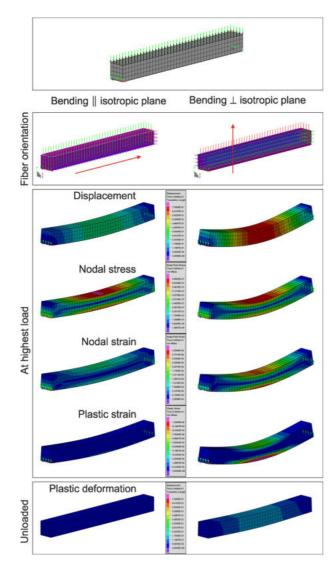
Figure 130: Transverse isotropic plasticity
