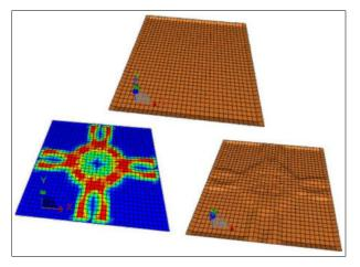
Figure 19: Bead design of a plate with positioning and height of beads
