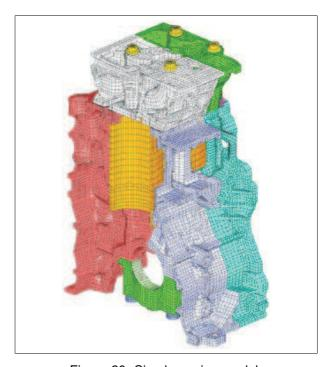
Figure 20: Simple engine model Daimler AG, Commercial Vehicle Division)
