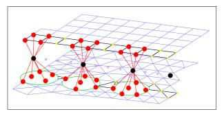
Figure 88: Connection of spotweld forces
