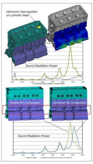
Figure 24: Optimization of rib thickness and rib position to reduce sound radiation from engine block surface
