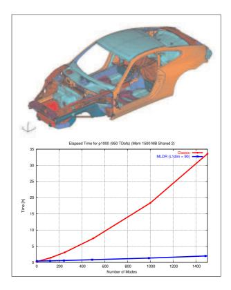
Figure 148: Comparison of elapsed run times for Subspace Iteration (upper curve) and MLDR (lower curve) with increasing number of modes (157412 Nodes, 164301 Elements (QUAD4), 944472 Unknowns)
