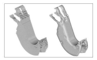
Figure 174: Layout-Optimization of a crane hook (on the left side the primary result, on the right side the smoothed surface)
