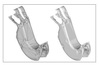
Figure 175: Polygon reduction (on the left side the triangle mesh, on the right side graphical representation of the surface)
