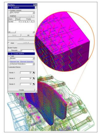
Figure 53: Material reference system for anisotropic material
