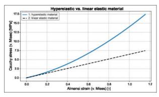
Figure 135: Hyperelastic material with non-linear relation between stress and strain (blue curve) and elastic material with linear relation between stress and strain (dashed curve)
