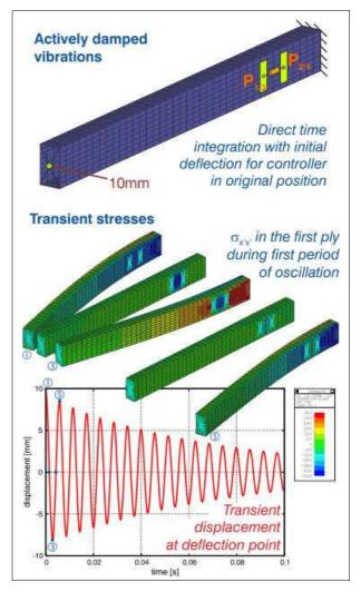
Figure 40: Active damping of a composite box girder
