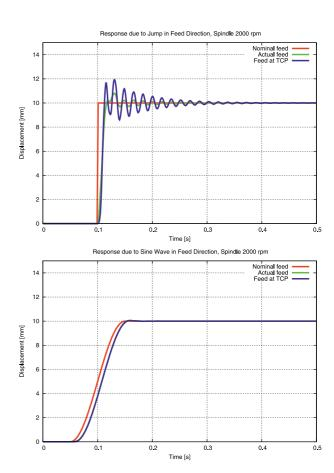
Figure 37: Time-history response due to excitation in Z direction for a sudden position jump (above) and a smooth position change (below) for the controlled machine
