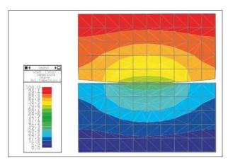
Figure 117: Temperature distribution in two contacting bodies
