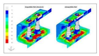
Figure 86: Results for part assembly with compatible (left) and incompatible (right) mesh
