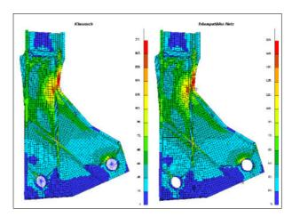
Figure 84: Ribbed shell model with compatible meshes (left) and incompatible meshes (right)
