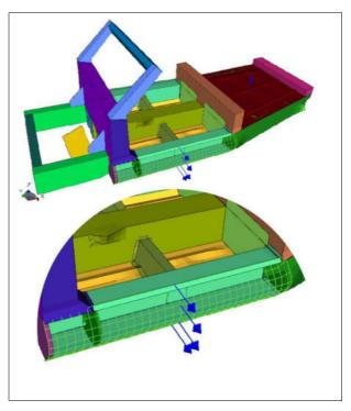
Figure 18: Shape optimization of a sill with transition to neighboured parts
