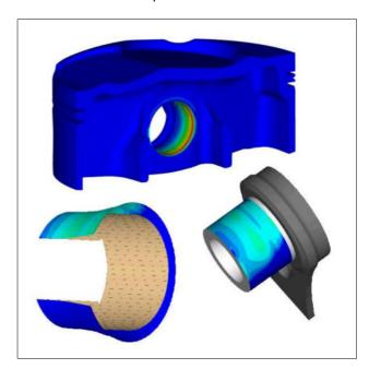
Figure 177: Optimization of contact pressure between piston and piston pin (Mahle GmbH, Stuttgart). The figure shows the optimized geometry of the piston and the reduced edge pressure.
