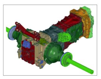
Figure 4: Model of a tractor transmission ZF Friedrichshafen AG, Friedrichshafen, Germany.
