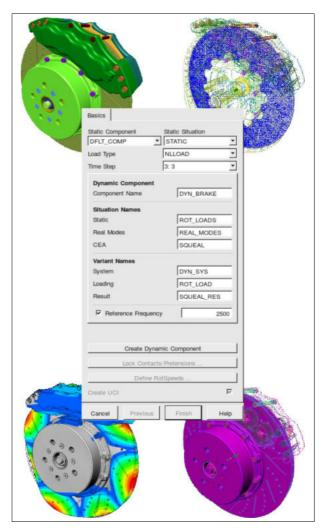
Figure 52: Preprocessing of brake models
