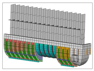
Figure 42: Optimization of a water box with 18 design variables and 19 stochastic basic variables
