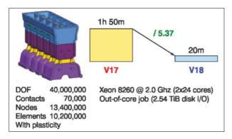
Figure 127: Parallel nonlinear element stress computation of a motor with 10.2 Mio elements
