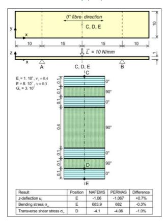
Figure 181: Laminate analysis of a *NAFEMS* composite benchmark.
