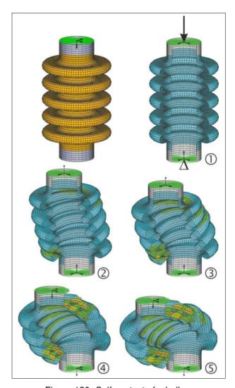
Figure 120: Self contact of a bellow
