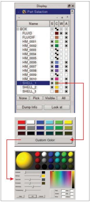
Figure 50: Graphics entities for parts and element groups (select S=Show, C=Colour, W=Wireframe, A=Active).
