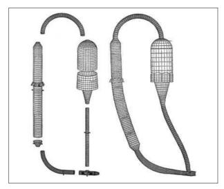
Figure 98: Mode shape of a reactor
