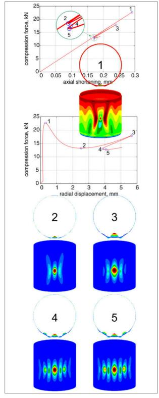
Figure 182: Nonlinear buckling with post-buckling behavior for a laminated cylinder shell
