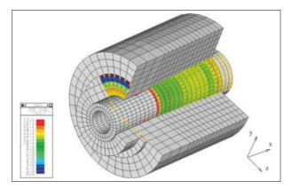
Figure 119: Conical *press fit* (slipping forces after assembly)
