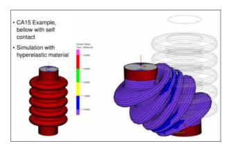
Figure 136: Bellow with self contact
