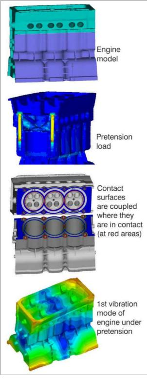
Figure 23: Dynamic analysis of an engine under pretension load
