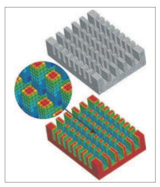
Figure 141: Analysis of cooling element with radiation
