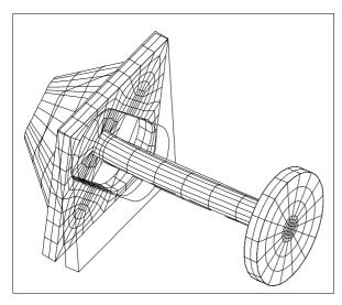
Figure 105: Clutch Element, Static Displacements
