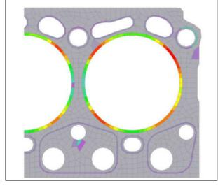
Figure 131: Pressure of cylinder head gasket
