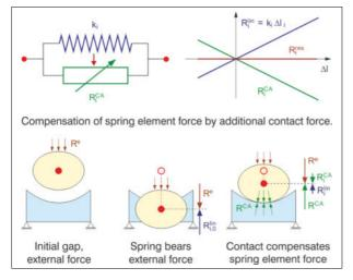
Figure 114: Force-guided contact with the aid of compensation spring
