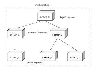
Figure 76: Substructuring in PERMAS
