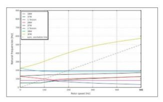
Figure 32: Campbell diagram for the evaluation of rotor dynamics
