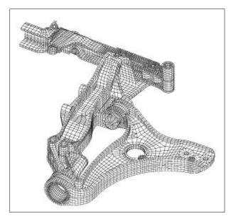
Figure 107: Model of a front axle Porsche AG, Weissach
