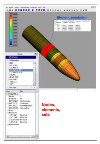
Figure 68: Checking element properties in a substructure model
