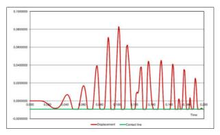
Figure 152: Transient response under contact conditions
