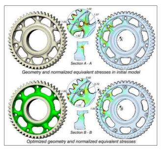
Figure 57: Shape optimization of a gearwheel Definition of cyclic symmetry, max. stress, minimum weight as objective function (by courtesy of Daimler AG, Stuttgart).
