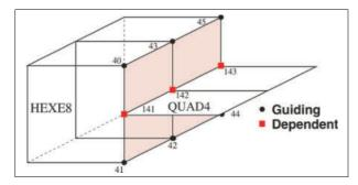
Figure 93: MPC example: Volume Shell Transition
