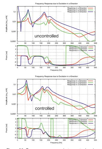
Figure 36: Frequency response between tool and workpiece due to excitation in Z direction for uncontrolled (above) and controlled (below) machine
