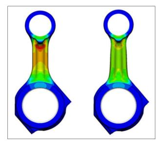
Figure 164: Stress homogenization of conrod
