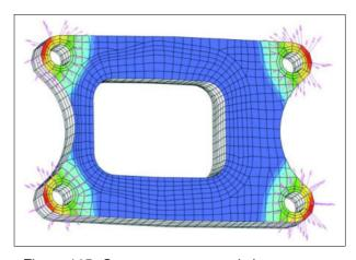
Figure 115: Contact pressure and shear vectors
