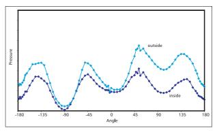
Figure 22: Pressure distribution at stopper over the angle
