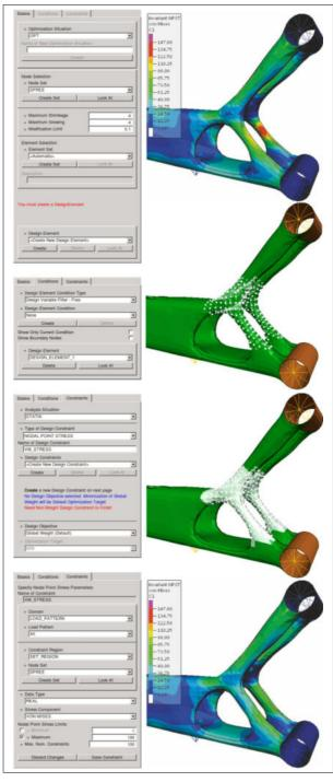
Figure 59: Pre- and post-processing for free-form optimization:
