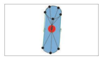
Figure 89: Spring element at spotweld position
