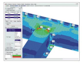
Figure 70: Evaluation of spotweld forces together with element stresses
