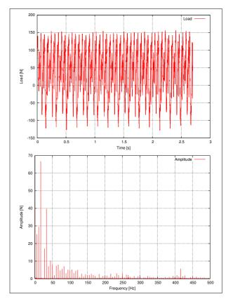
Figure 100: Example for the transformation of a periodic load (above in time domain, below in frequency domain)
