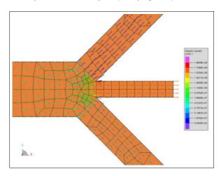
Figure 185: Electric current in an electric junction
