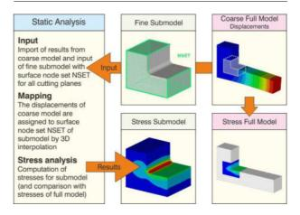
Figure 77: Submodeling in static analysis
