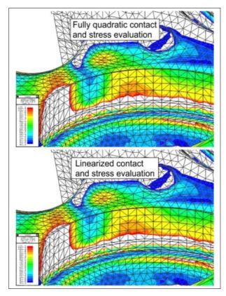
Figure 116: Nodal point stresses on surface with linearization (bottom), and without linearization as reference (top).
