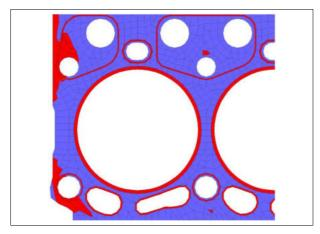
Figure 21: Contact status for gasket elements
