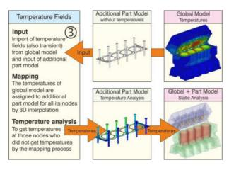
Figure 79: Mapping with extrapolation of temperature fields
