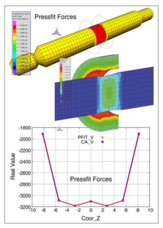
Figure 94: Press fit between shaft and hub Identical stress results of MPC and contact solution.
