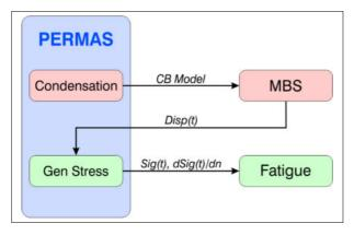
Figure 167: Use of MBS and Fatigue coupled to PERMAS.
