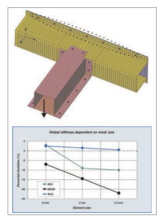
Figure 183: Quality of the refined weldspot model
