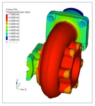
Figure 139: Temperature field of a turbocharger
