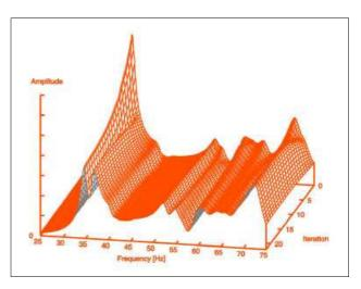
Figure 162: Iteration history of a frequency response optimization
