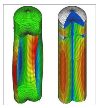
Figure 156: A coupled vibration mode shape of a fluid-filled space tank with corresponding pressure mode
