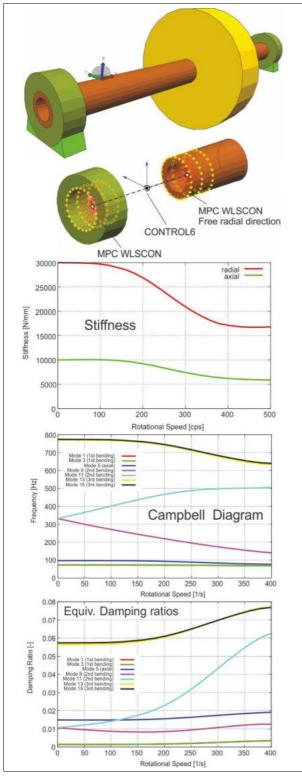
Figure 146: Rotor with rotation speed dependent supports
