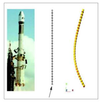
Figure 184: Displacements of flying rocket under thrust and dead weight.
