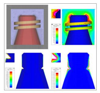
Figure 186: Example for electrodynamic induction, model and magnetic field strength (top), induced heat flux and plastic strains (below).
