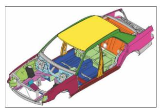
Figure 159: Frequency response optimization of a body-in-white with shape and sizing parameters (see also Fig. 162)
