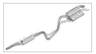
Figure 188: Mode Shape of an Exhaust System
