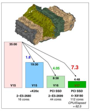
Figure 118: Contact analysis of an engine with 56 Million DOF, 37 time steps, 2 different temperature states, and CAS files, direct I/O with PCI SSD.
