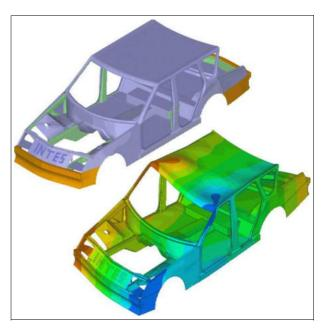
Figure 17: Workshop example INTEScar under torsional loading
