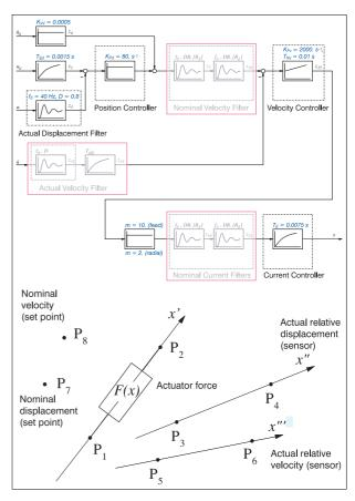
Figure 35: Block diagram of used controller and corresponding finite element representation
