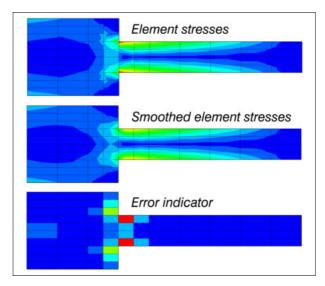
Figure 97: Element stresses, smoothed element stresses, and absolute error indicator
