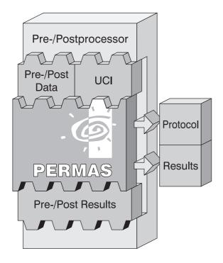
Figure 102: Integration of PERMAS in pre- and post-processor
