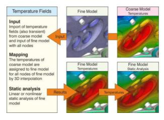
Figure 78: Mapping of temperature fields
