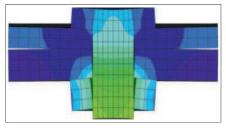
Figure 25: Short bolt under pretension
