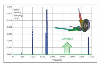
Figure 31: Stability map of a brake for 7110 parameter sets from rotational speeds, Young's modulus of disk, and frictional coefficient between disk and pad. The total run time for this stability map was 5 hours 12 minutes.
