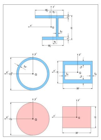
Figure 96: Standard beam cross sections
