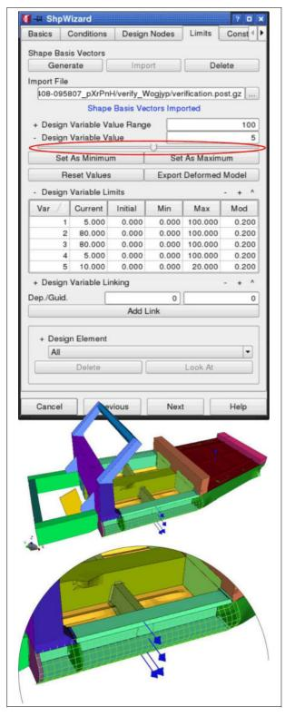
Figure 58: Definition of shape basis vectors of a car sill. The shape changes can be visualized by moving the slider in the menu.
