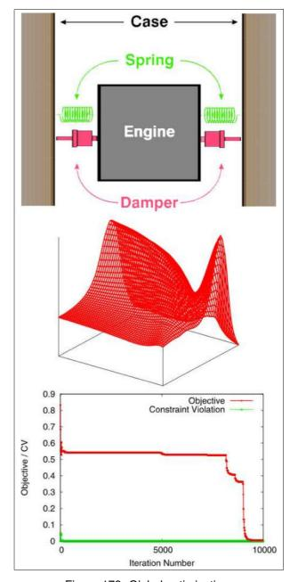
Figure 178: Global optimization of a spring-damper system with the LDR method. Top: model with 4 design variables, Middle: 2 design variables fixed at the optimum, objective function dependent on the 2 free variables, Bottom: course of objective function and constraint violation during the iterations.
