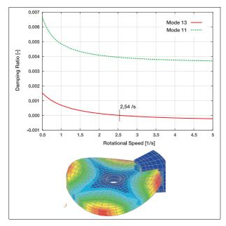
Figure 27: Simple brake model (1) with an unstable bending mode (m=2, n=1) at 2,54 rps
