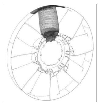
Figure 81: Cyclic symmetry of a fan Behr GmbH & Co., Stuttgart, Germany.
