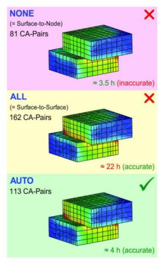
Figure 109: Surface-to-surface contact with COMPLEMENT option: Best compromise between accuracy and computation time (von Mises nodal stresses are shown). The numbers are taken from an industrial application.
