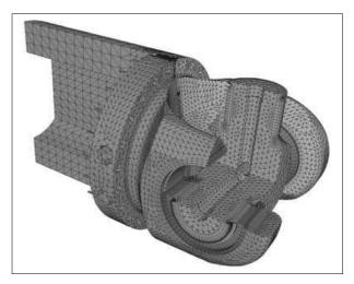
Figure 82: Incompatible meshes Cardan shaft model in sectional view (Voith Turbo GmbH & Co. KG)
