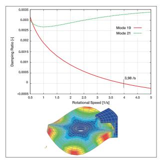
Figure 28: Simple brake model (2) with an unstable bending mode (m=3, n=1) at 3,98 rps
