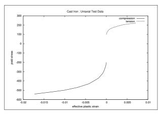
Figure 133: Uniaxial test data of a cast iron material
