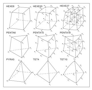
Figure 134: Large strain elements
