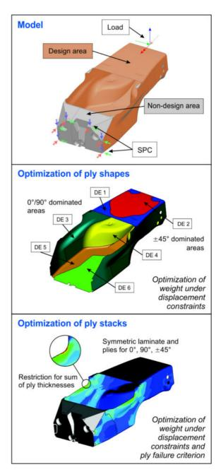
Figure 168: Optimizing laminates for a racing car monocoque with free sizing (see 107) to get a thickness distribution of the layers and with sizing (see page 100) to optimize ply thickness and angle.
