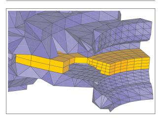
Figure 83: Incompatible meshes Element transition (HEXE8/TET10)
