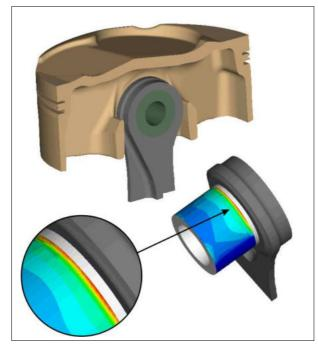
Figure 176: Optimization of contact pressure between piston and piston pin (Mahle GmbH, Stuttgart). The figure shows the edge pressure between both parts (for the optimized result see also next Fig. 177).
