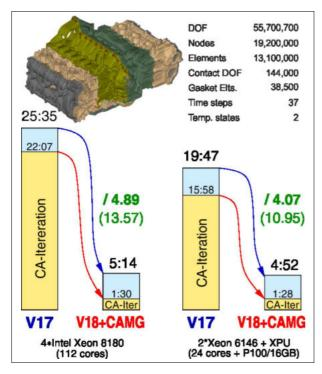
Figure 122: Contact analysis of an engine with 56 Million DOF, 37 time steps, 2 different temperature states
