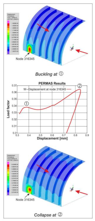
Figure 129: Elastic-plastic buckling with post-buckling behavior
