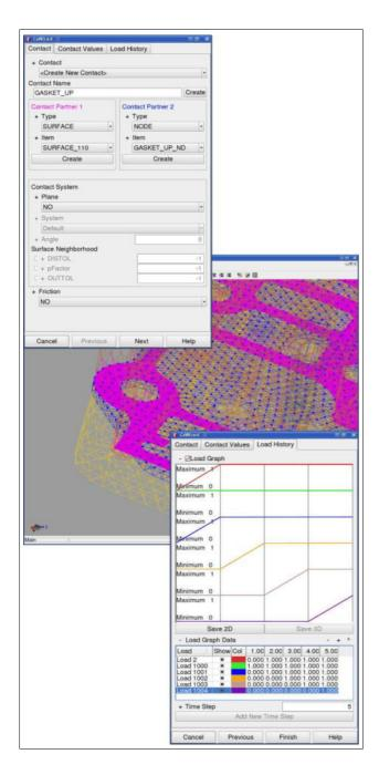
Figure 64: Contact modeling Contact topology and load history definition
