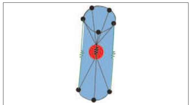
Figure 113: Spring element at spotweld position
