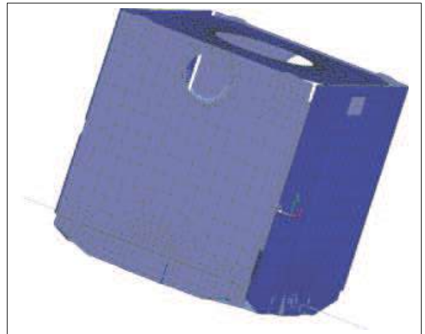
Figure 60: Optimization of PROTEUS satellite with 28 design variables and 30 stochastic basic variables (Alcatel Space S.A.)
