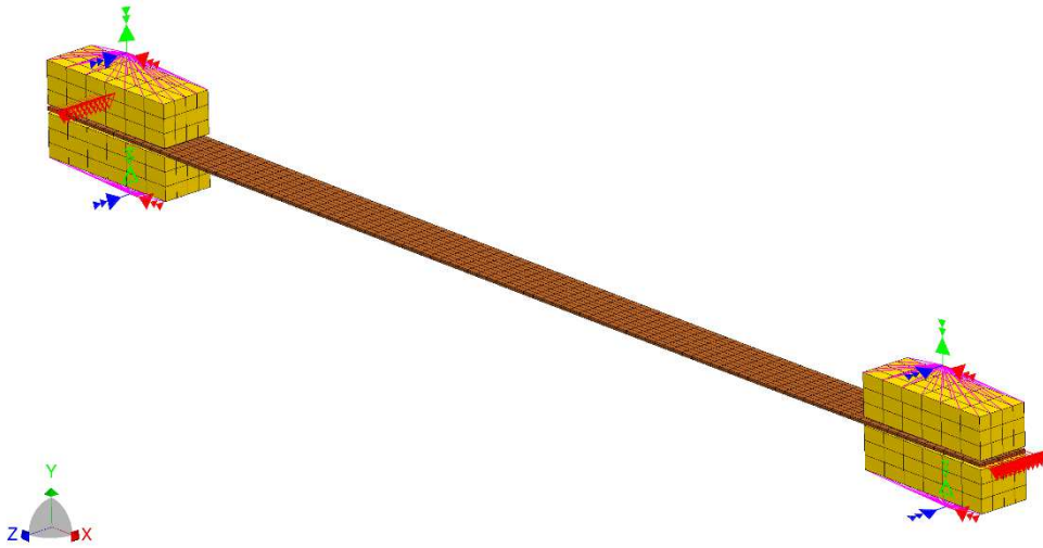
Figure 1: Finite element model of the clamping fixture and beam
