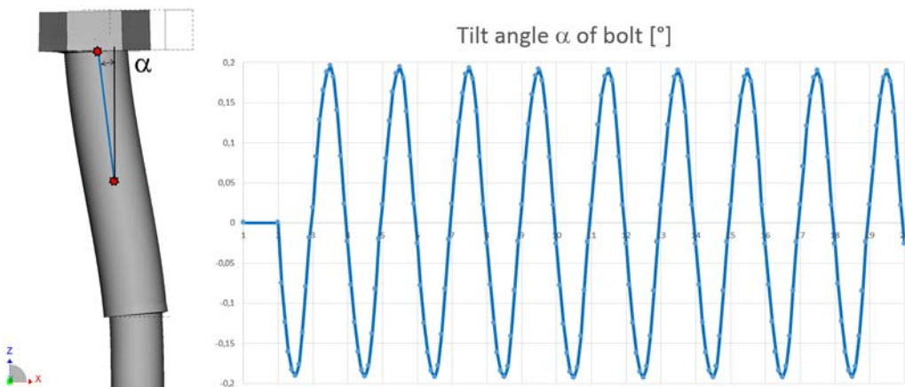
Figure 4: Tilt angle of bolt (displacement scaled by factor 50) and behaviour during FE-analysis
